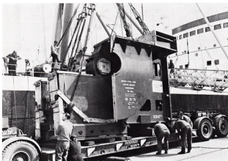
■ B&C vessels continue to get their share of heavy lifts. In the pictures above, left and right, Clan Macilwraith uses her own gear to discharge a 60-ton piece of machinery onto one of Pickfords low loaders. The massive item was destined for the British Steel Corporation's Anchor Project in Scunthorpe, and was manufactured by the Broderick Engineering Works Ltd. Pictures: S. D. Trumper, Hull.
