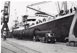
■ At right and below, two king-size lifts for King George in Genoa recently. At right, positioning a boiler, weighing 50 metric tonnes, prior to lifting. Below, using the ship's own gear to load a cracking tower unit weighing 30 metric tonnes and measuring 104 feet 4 inches long. In the shot below right, taken from a neighbouring roof, the tower is seen being settled into its deck position. Both items were part of the Ndola oil refinery and were destined for Beira, Mozambique. Pictures below by Capt. J. D. W. Chapple; at right by radio officer J. Braddock.
